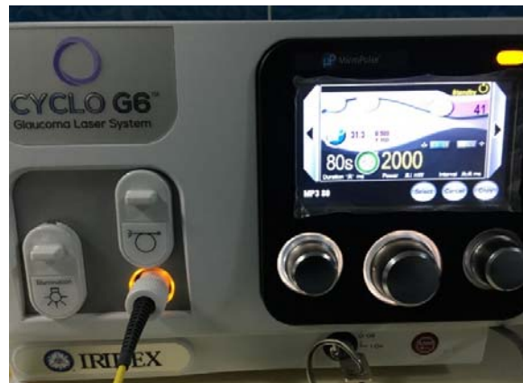
Figure 2. The Cyclo G6 diode micropulse system set to 31.3% duty cycle and 2W power.
