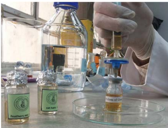
Figure 2. Secondary filtration of the allergenic extract using Millipore Syringe Filter.
