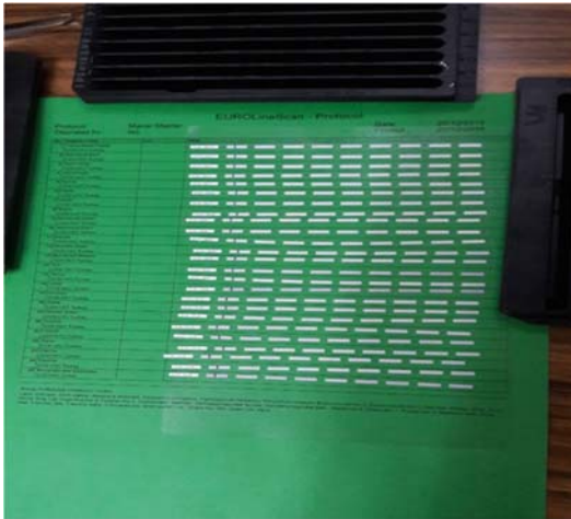
Figure 5. Test strips placed on the evaluation protocol ready for digital evaluation.
