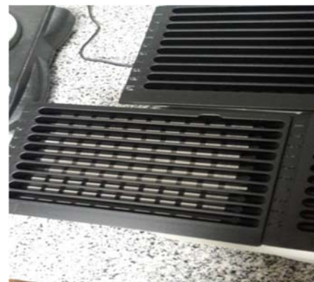
Figure 4. Test strips coated with allergens in the incubation tray.
